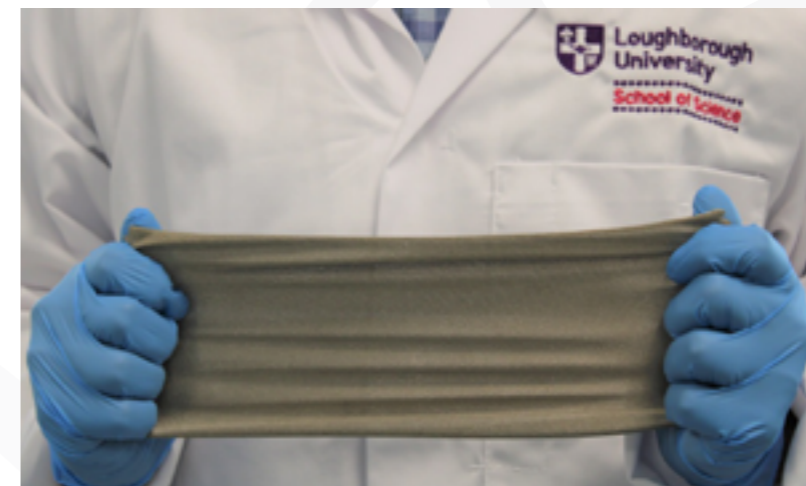
Pictured is the lightweight and thin TENG textile that produced over 35V of voltage using mild artificial movements. It could potentially power low-power health sensors, environmental sensors, and electronic devices in the near future.
